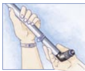
Assembling Poly Pipe: 1. Place clamp over pipe, then insert barb fitting.
