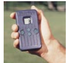
SRR Remote Control Kit The Hunter SRR Remote Control Kit saves time during installation and routine system maintenance. The receiver (left) plugs into the Controller Connection Kit and the transmitter (above) activates the sprinklers within a 450' range. The user can manually run any zone without resetting the controller.
